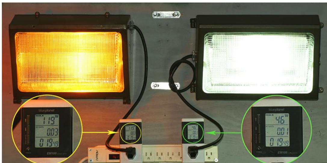
**Wallpacks:** This photo shows a side-by-side comparison of Wallpack fixtures commonly used on the exterior of buildings as security/perimeter lighting.
