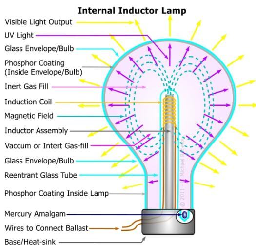
Internal Inductor lamps typically consist of a light bulb shaped glass lamp, which has a test-tube like central re-entrant cavity (glass tube) in the center, and where the interior is coated with phosphors and filled with inert gas, with a pellet of mercury amalgam usually located in a tubule at the bottom of the lamp (see diagram on left).
