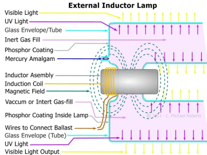
External inductor lamps are basically fluorescent lamps with magnetic induction coils wrapped around a part of the outside of the tube. The interior of the tube is coated with phosphors, and has a small pellet of mercury amalgam usually located in a tubule near the inductor (see diagram on left).
